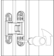
Raise or lower the door by adjusting the (air) wedge. Alternatively, the door can be raised by inserting and turning a flathead screwdriver in the slotted section.
