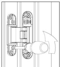
To adjust the door in depth, loosen all four screws on the flange side 180° in counter-clock wise direction with a screwdriver.
