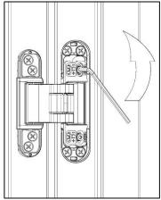
Support the door with a (air) wedge. Loosen both outer height adjust screws of each hinge 1 turn of 360° with a hex-key.
