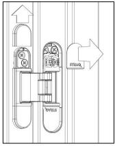
Remove the four screw covers from the hinge before adjusting the hinge and door.
