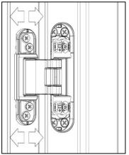
Manually adjust the door element toward the desired depth position.
