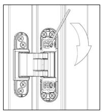
To increase the gap between door and doorframe, turn inner +/- screw clockwise 2x360° with a 3mm hex key.
