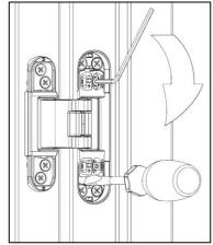
Secure the door by tighten both outer height adjust screws of each hinge in clock wise direction with a hex-key.
