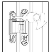
Secure the door by tighten all four screws in clock wise direction with a screwdriver.
